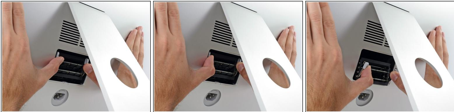
**i** The RAM tray is locked into its upright position with two grey tabs.
